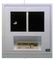
designed to overcome potential infection control issues and create more space in the operating theatre. They can be flush mounted into the wall of the operating theatre (w-PACS) or the surgeons control panel (r-PACS) or can be a mobile viewing station (m-PACS).
