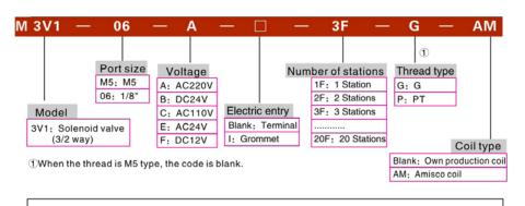
The above codes have included the series accessories, so it is unnecessary to order the accessories specially. But if you like, you could order as follows. Code of accessories | Accessory name Part code Part name Quantity F-3V1002N Coupling screw(S) 3V1-P30 Coupling screw assembly F-3V1003N Coupling screw(M) 2 GOR20008N75 O-Ring 1 3V1-P31 Coupling screw assembly F-3V1004N 2 Coupling screw(L) F-3V1001N Fixed mounting 3V1-P32 Bracket assembly GSDA04008WA Cross round head screw
