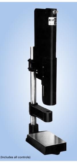
AH-65 delivers a consistent, uniform blow. It is designed to accelerate, then strike a tool which may be guided by the supplied tool arm. A spring returns the hammer to the start position after the work is completed. The head must be free with no fixturing or tooling attached directly to it.
