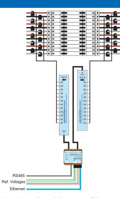
In situations where it is not possible to mount the carrier strip adjacent to the pan assembly C-Matic Systems offer the SPLIT CT SPN. This solution is particularly suited to enhancing existing PDUs with final circuit monitoring. The carrier strips containing the nodes can be mounted along with the intelligent link controller at a convenient location. Each node uses a remote split core CT that can be attached to the circuit of interest.
