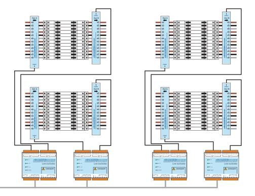
Note: Each Intelligent link controller and Intelligent Marshalling Unit can be interfaced to a maximum of 48 nodes.
