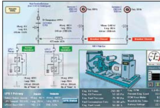
Example screen from PowerLogic ION Enterprise software showing electrical system diagram with multiple real-time metering points.
