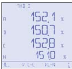
Current total harmonic distortion display
