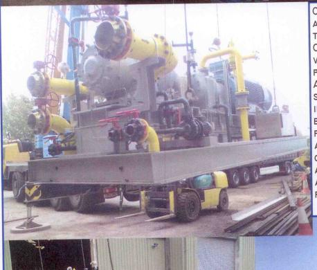
OUR INVOLVEMENT IN PRESSURISED PIPE AND VESSEL PROJECTS CONTINUED WITH MANUFACTURE OF COMPRESSOR UNITS AND A FILTRATION FOR VESSEL PACKAGE PETRO-CHEMICAL INDUSTRY. BUILT TO PD5500 B31.3 AND SPECIFICATION INCLUDING INSPECTION, PRESSURE TEST TO 18 BARG AND 30% ULTRASONIC NDT. AS PART OF THE CONTRACT WE DEVELOPED A FULL 3D PROJECT MODEL, CARRIED OUT STRUCTRUAL AND VESSEL DESIGN AND FABRICATION DETAILS AS WELL AS ASSEMBLY AND TRIAL RUNNING OF THE PLANT.
